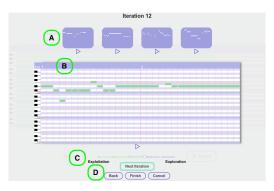
Figure 2: Interface for the search. (A) Current candidate melodies that BO sampled. (B) Editing widget. (C) Slider for specifying the exploration-exploitation balance for the next iteration. (D) Buttons to control the workflow.
